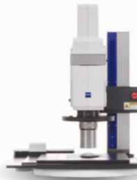
ZEISS Axio Zoom.V16 For particle size \geq 5 \mu\text{m} Recommended for extended analyses
